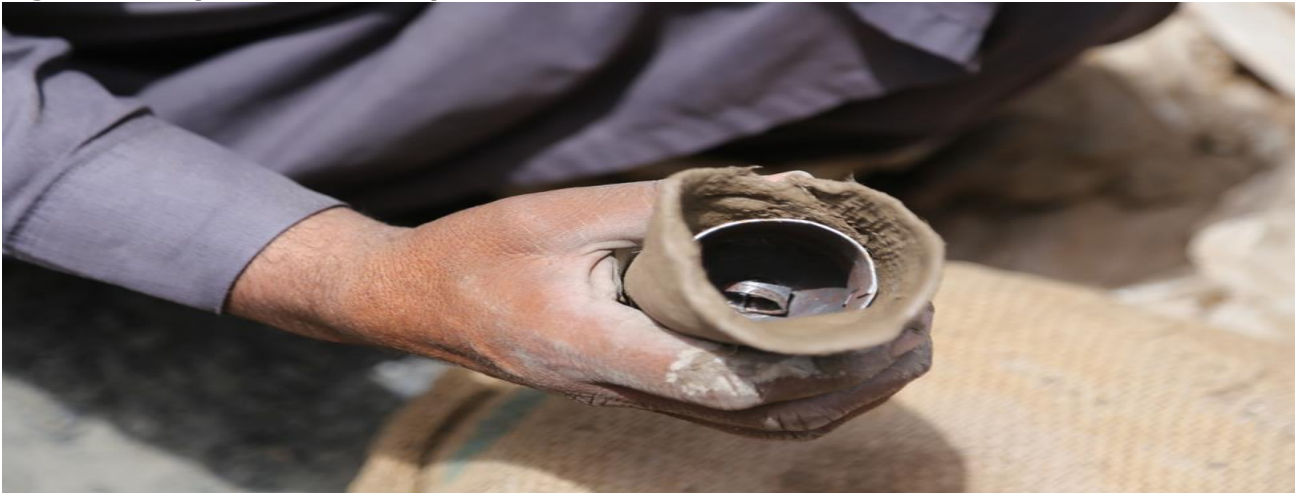
Figure 6: Clay is used to wrap the iron bells
