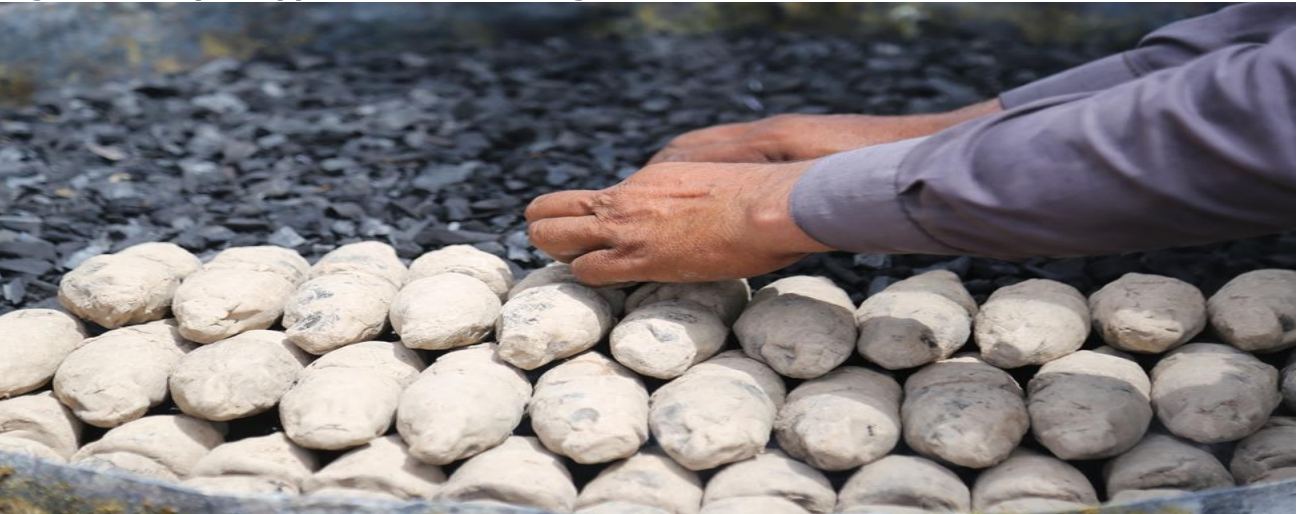
Figure 8: Clay wrapped iron bells being baked in the coal fueled kiln
