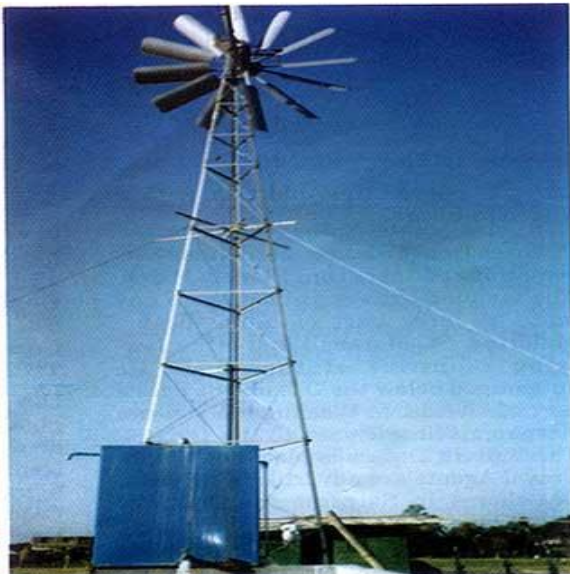
Figure 2: A Wind Pump at Patenga, Chittagong
